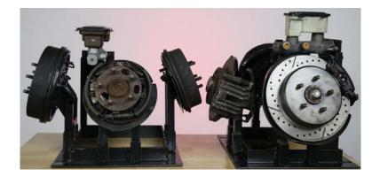
With this compact, customizable training aid, an instructor doesn't need to put a car on the lift to demonstrate automotive brake system operations or repairs.
