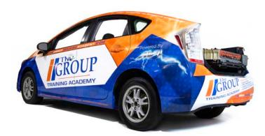
AVI's Hybrid Electric Cutaway Vehicle Trainer is a fully operational vehicle developed for static and active training scenarios. There are secondary, de-energized high voltage components such as an additional battery, inverter, and motor generator for introductory practical exercises.
