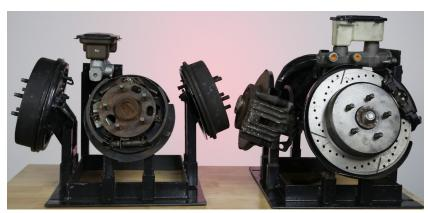
With this compact, customizable piece of training equipment, an instructor dosen't need to put a car on the lift to demostrate brake system operations.
