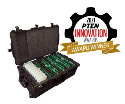
The ATS Tools: eTRAINER JR hands-on training simulator will cover the operation and testing of basic to advanced electronic circuits. This training program provides the student with a complete step-by-step coursethat will enable the student to understand what the voltage measuring instrument is conveying to the technician.
