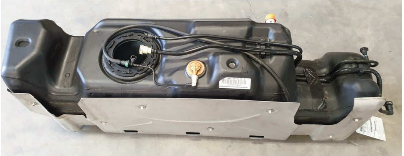
Duramax L5P Primary Fuel Tank
