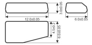
The new physical shape will not affect performance or vehicle applications that are covered. Ilco will continue to refer to this transponder as the GTI. The new physical shape will continue to fit into the GTH head and GTS Look-Alike shells. This is simply a rolling change. Any existing inventory of glass tube GTI transponders will continue to work as usual.
