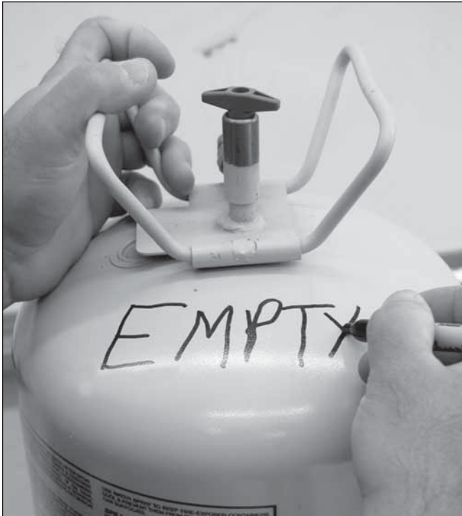
Empty refrigerant cylinders should be marked "Empty" before disposal.
