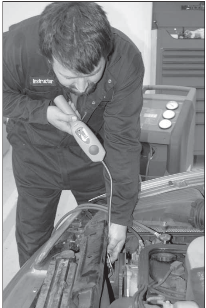
Your electronic leak detector(s) must be certified to meet the SAE spec (the detector should be labeled as such), and must be used in accordance with the procedures outlined in the SAE J1628 spec. We've provided an overview of J1628 under “Using Electronic Leak Detectors,” (this page) and in the sidebar on page 19.
