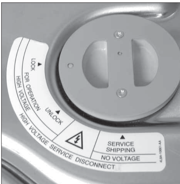
Example of a high voltage disconnect device on a hybrid vehicle. When performing service on any hybrid or electric vehicle, ALWAYS follow the vehicle manufacturer's recommended safety procedures.
