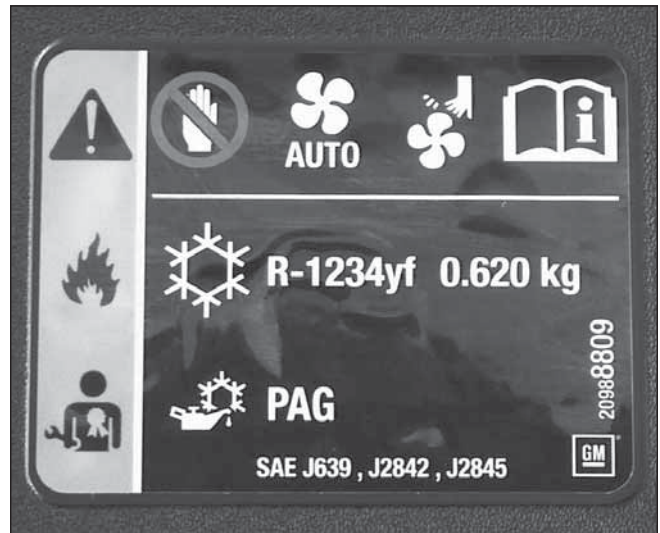
Label used on the 2013 Cadillac XTS, the first GM car to use the new refrigerant.
