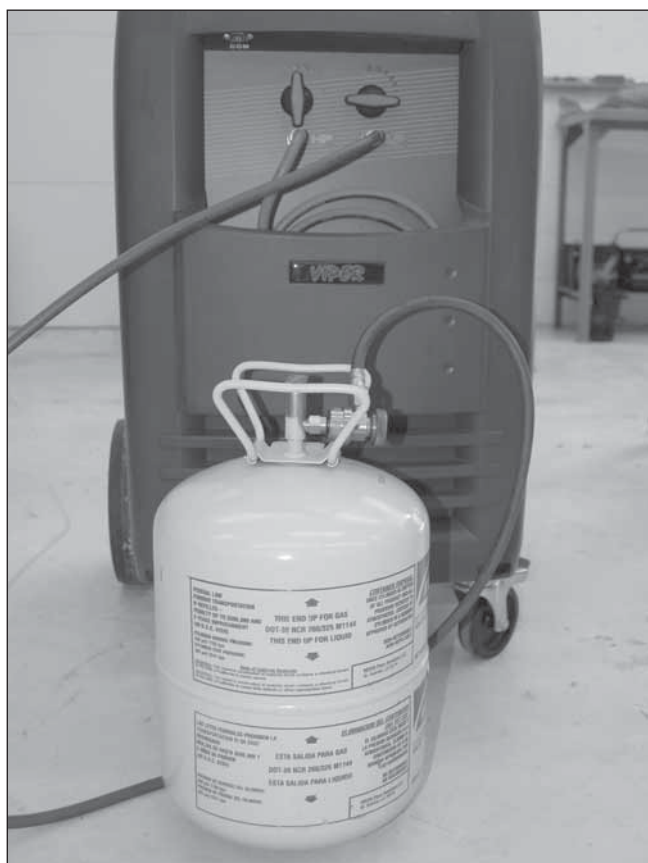
Before they are discarded, disposable refrigerant cylinders should be connected to recovery equipment and brought to a vacuum. This will ensure that all refrigerant has been removed.
