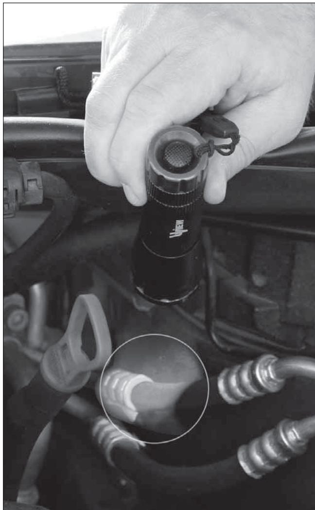
The leaking dye will glow under ultraviolet light. (Courtesy GPS Automotive Group)
