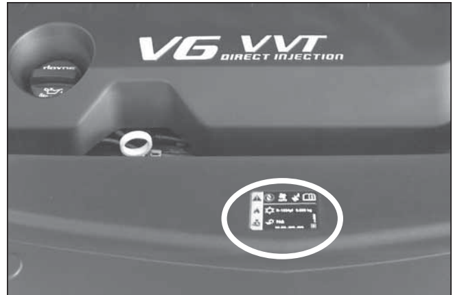
The refrigerant label is easy to find on the 2013 Cadillac XTS but you may have to look around on other vehicles.
