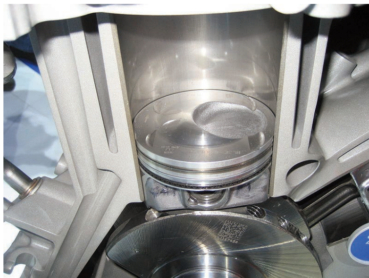
PISTON OF A 3.5 L (210 CU IN) FORD ECOBOOST ENGINE WITH A SWIRL CAVITY ON THE TOP
