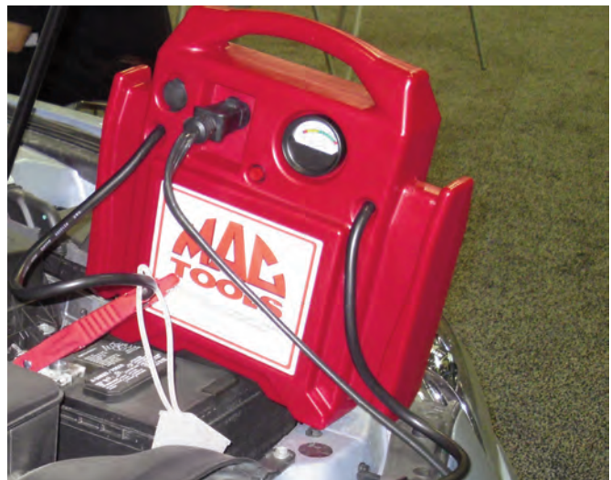
When charging or using a battery booster pack, always connect the terminals and then turn on the machine.
