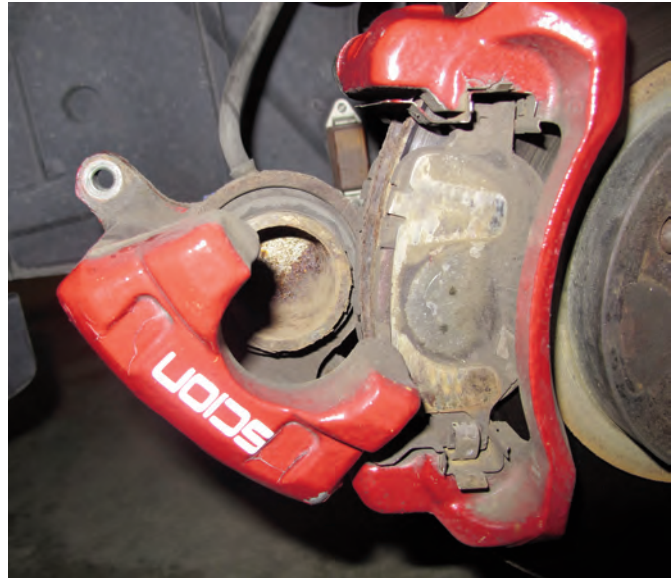
Fig. 18 With floating calipers, the anchor plate attaches to the chassis, and the caliper body slides on guide pins connected to the anchor plate as the brakes are applied. To replace the pads, the caliper body must be separated from the anchor plate.
