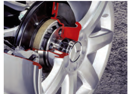
Photo 5 Rear rotor with the parking brake in the hat.
