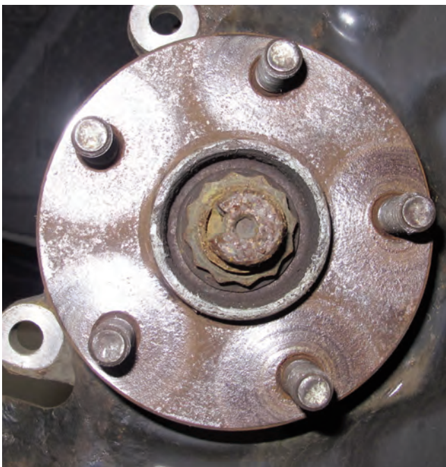
Photo 7 Clean the hub flange to prevent runout issues.
