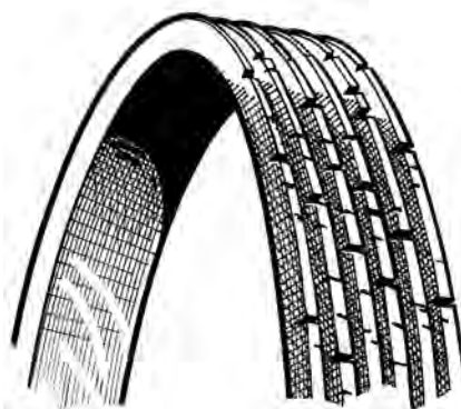
Belts should be free from cracks and glazing.
