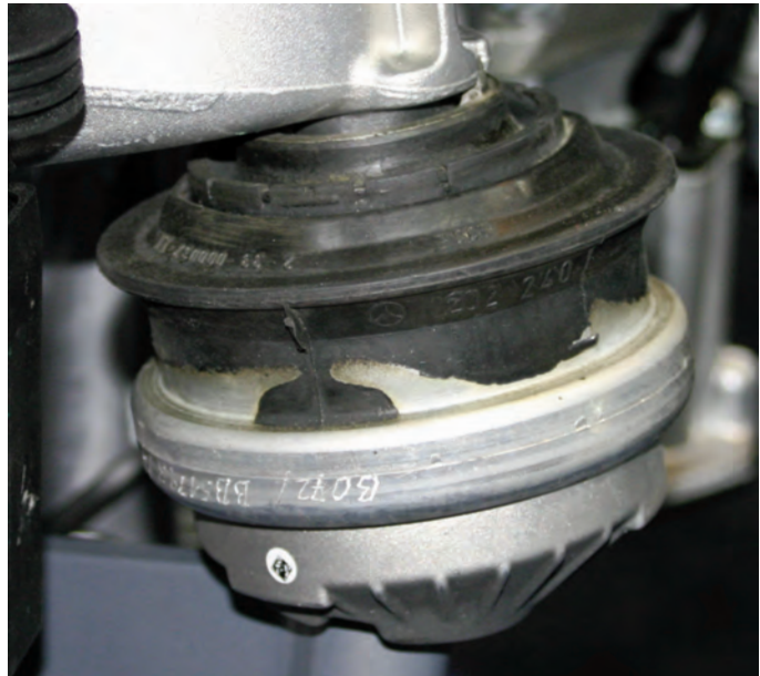
If an engine mount is leaking oil, it is a sign of a failure of the mount.
