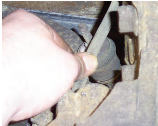
Photo 1: Always inspect brake hoses for crimps, bulges and defects.
