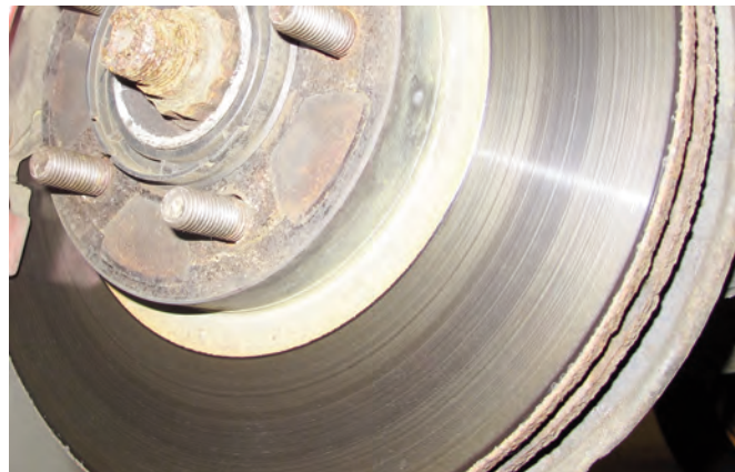
Photo 3 Pad material transfer on a rotor.
