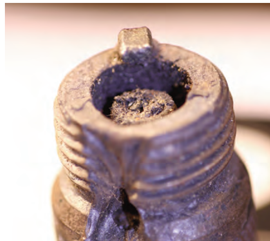
Pre-ignition and knock can damage the spark plug.
