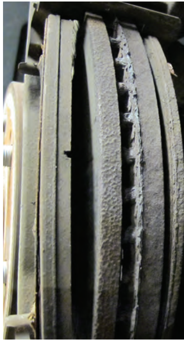
Photo 2: Uneven brake wear is a sign the caliper is seized
