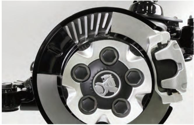
Photo 4 Spiral rotor fins on a vented rotor.
