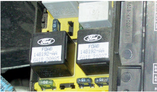
The starter solenoid is often controlled by a relay. The relay is typically controlled by the engine control computer.
