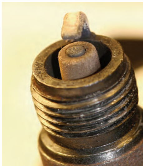
Worn out spark plug with a large gap.
