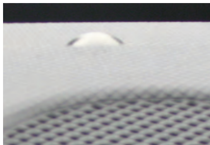
Vehicle with automatic temperature control measure the interior's solar load in order to determine blower and compressor settings.
