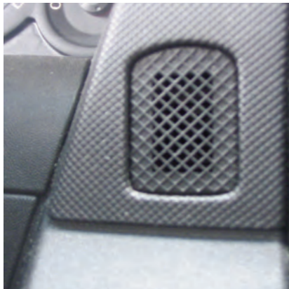
Vehicle with automatic temperature control measure the interior's ambient temperature. Behind the screen is a small fan and a temperature sensor.
