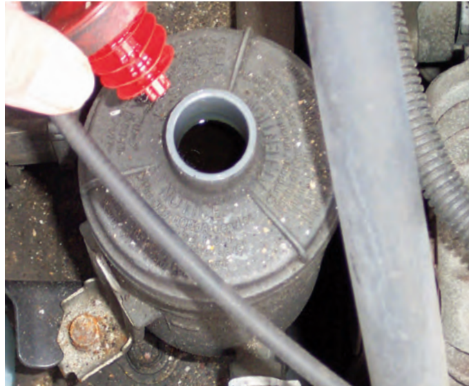
Often the reservoir will have the required fluid imprinted on the top or on the cap. If it can not be found, check the owner's manual or a fluid supplier's catalog.
