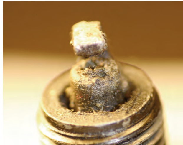
Pre-ignition can be caused by carbon deposits in the combustion chamber.
