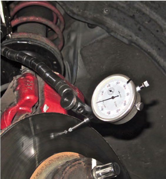
Fig. 8 Dial indicator setup to measure rotor lateral runout.
