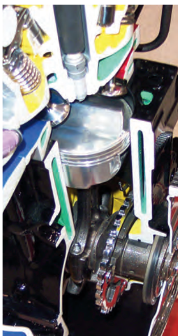
Oil from the crankcase and connecting rod lubrication holes can be sucked into the combustion chamber if the piston rings are worn. Also, coolant from a leaking gasket can be ingested.
