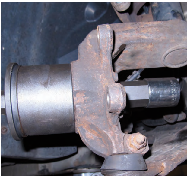
The sealed wheel bearings on some FWD vehicles are press fit to the hub and steering knuckle, so the steering knuckle must be removed from the vehicle to service them.
