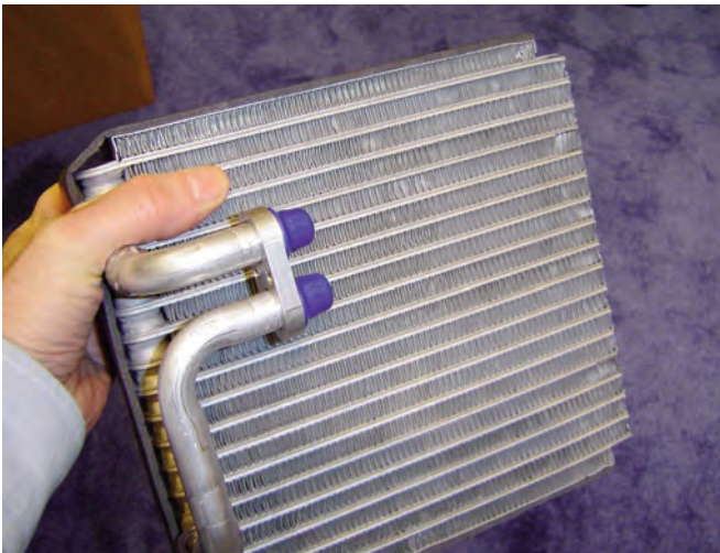
The evaporator core is located inside the vehicle and cools the air. It is also used to remove moisture from the air used to defrost the windows.
