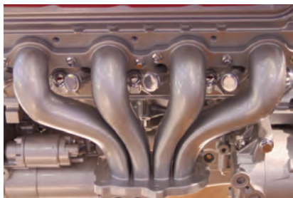
The exhaust manifold or header, must be free of defects so it seals.
