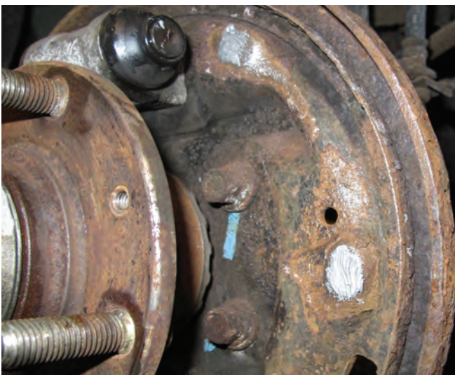
Apply a thin coat of high-temperature brake grease to the shoe contact pads on the backing plate.
