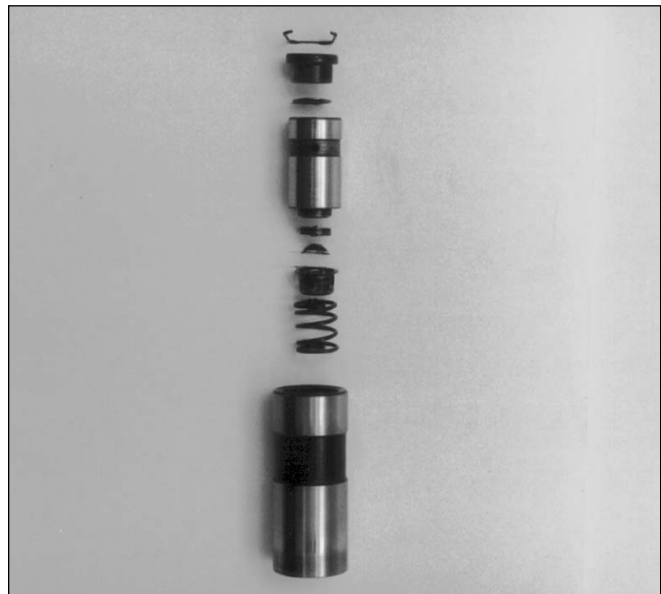
Fig. 2-31. Most hydraulic lifters can be disassembled for cleaning and inspection.
