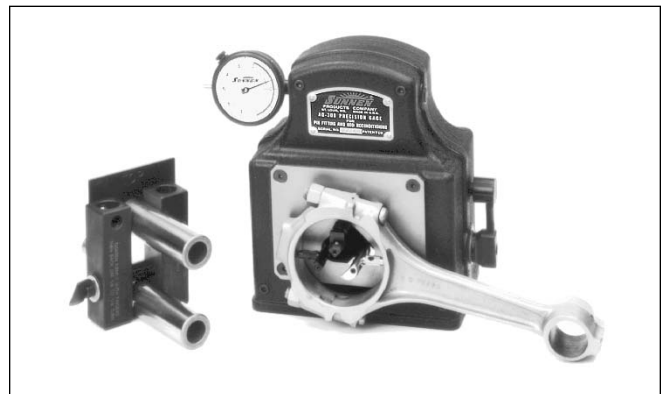
Fig. 3-28. A precision bore gauge can be used to measure connecting rod bores.
