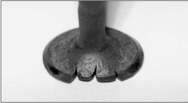
Fig. 2-17. Valve burning and guttering results from overheating.
