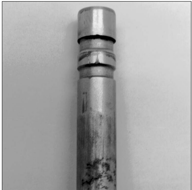
Fig. 2-20. Check for scoring or galling on the valve stem and for signs of stress at the tip end.
