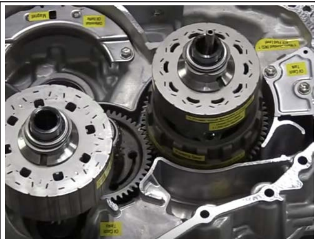
Gear Train Parallel Design
