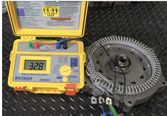
EXTECH Digital Milliohm Meter - Rotor Testing
