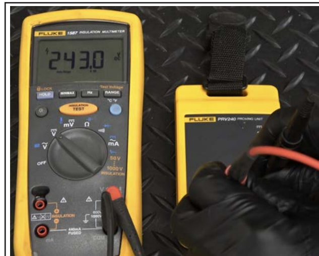
Fluke CAT 3 Meter and PRV240 in use
