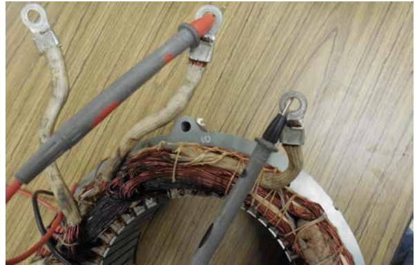
Motor Short Testing
