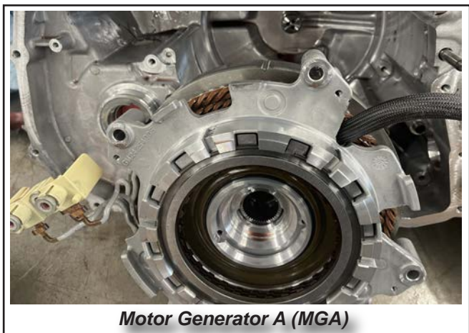
Motor Generator A
