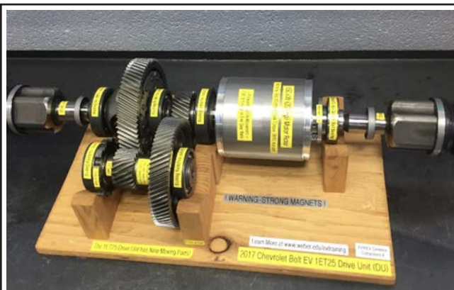
Chevrolet Bolt EV 1ET25 Gear Assembly
