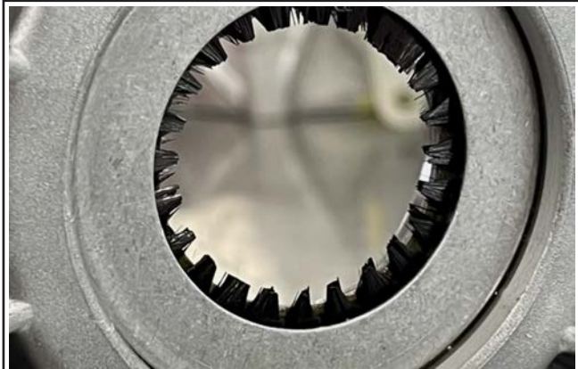
Tesla Grounding Strands
