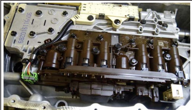
GM 6L90 Transmission (internals)
