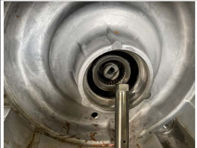
Gen 2 Oil Pump Drive Shaft (removed)
