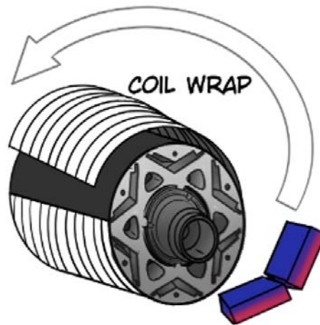
Tesla IPMSynRM Coil Wrap
