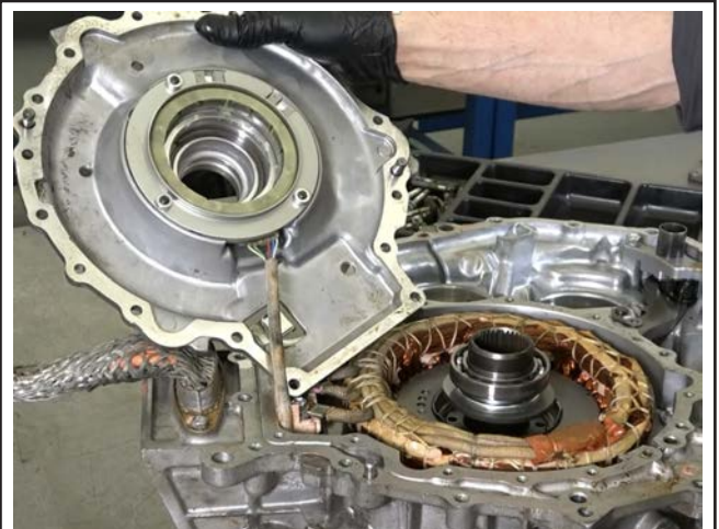
Access to MG1
