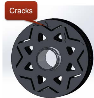
Rotor Failure (cracking)
