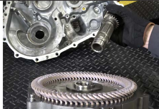
Rotor and Shaft (Removed)
