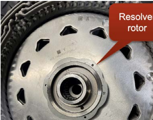
Six Sided Resolver Rotor
