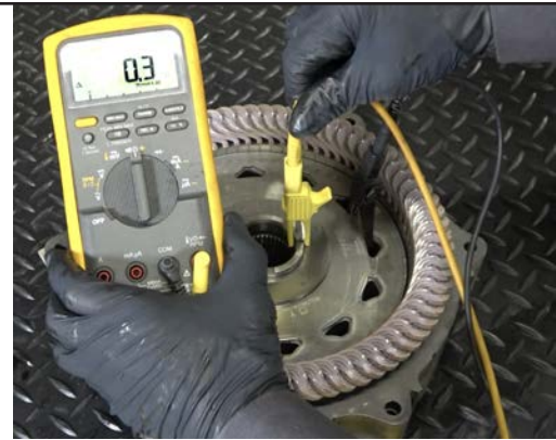
Honda Dual Motor Rotor Current Test
