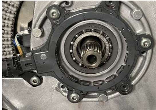
Honda Dual Motor Rotor Shaft Bearing Assy.
