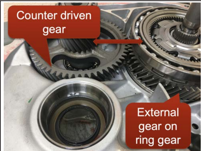
Counter Driven Gear and External Gear (ring gear)
