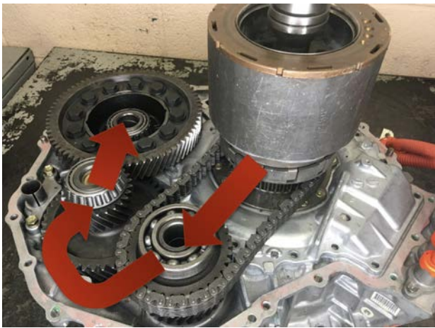
First Generation HSD Cutaway (power flow)
