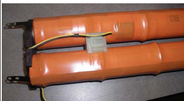
Batteries Welded Together in Series
