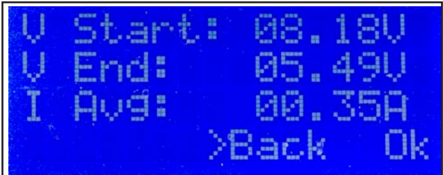
Capacity Test Failure
