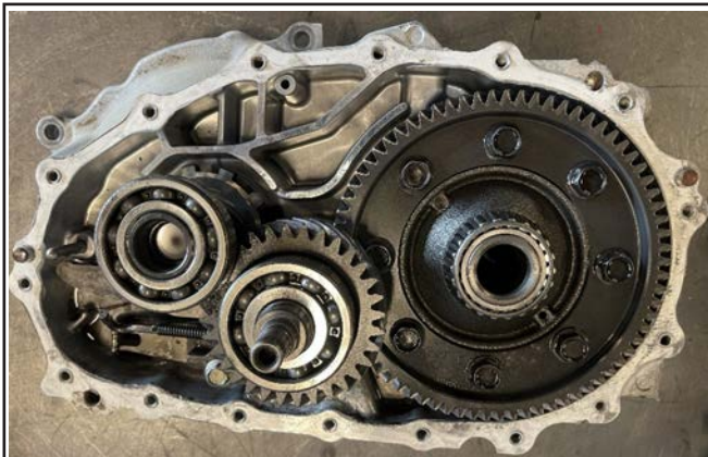
Nissan Leaf BEV Compound Gear Assembly
