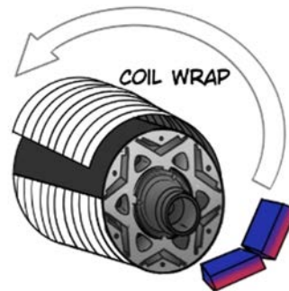
Tesla High-Speed Rotor
